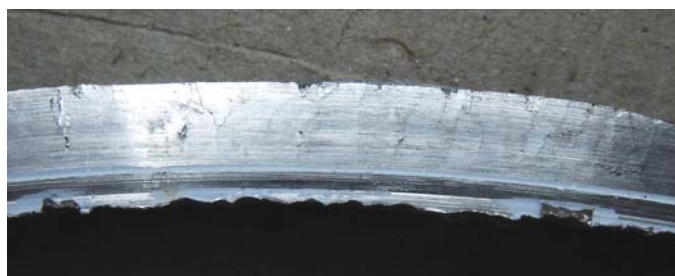
Figure 3. Cross section of the middle of zone with the highest cracking density.
