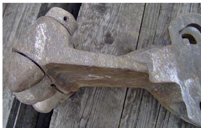
Figure 8. Wear of the scrapers. Slika 8. Trošenje strugača
