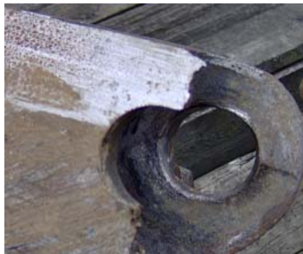
Figure 4. Wear of the chain elements by micro cutting.
