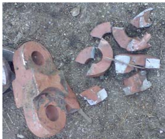
Figure 9. Fracture of chain elements (connecting chain links). Slika 9. Lom elemenata lanca (vezne karike)
