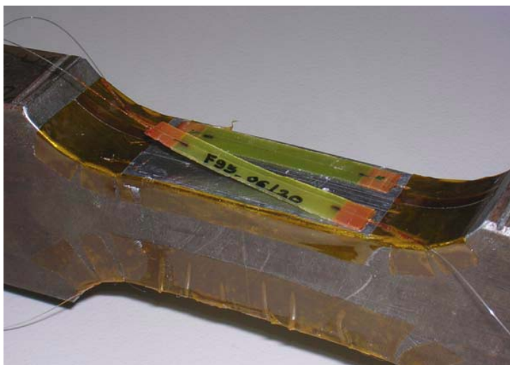
Figure 8. Optical strain gauge at clamp, applied strain 3 000 \mu\text{m}/\text{m} .
