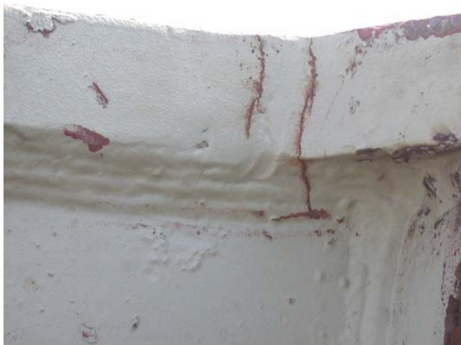
Figure 2. Cracks on the mast of BWE.
