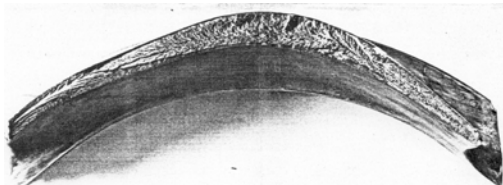
Figure 20. Brutal fracture of blade due to overloading, /27/.
