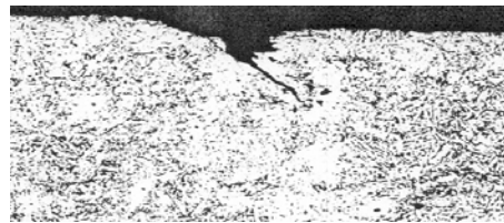
Figure 22. Corrosion attack at blade surface, /27/.
