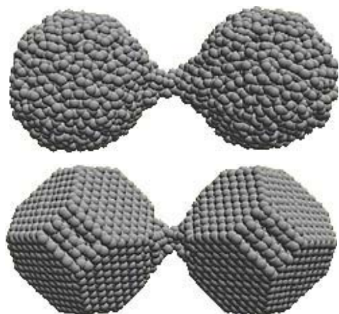
Figure 40. NIST researchers have shown that silica that are brittle in bulk, exhibit ductile behaviour at the nanoscale. Computer simulations demonstrate material extension and necking that occurs during the separation of amorphous (top) and crystalline (bottom) silica nanoparticles, /59/.
