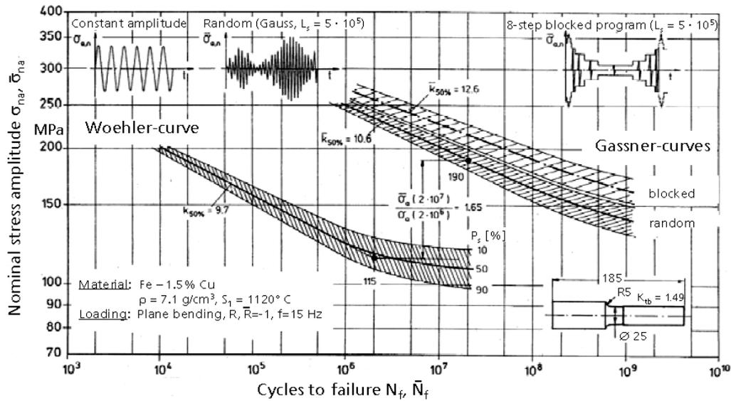
Figure 14. Influence of load sequence arrangement on fatigue life.
