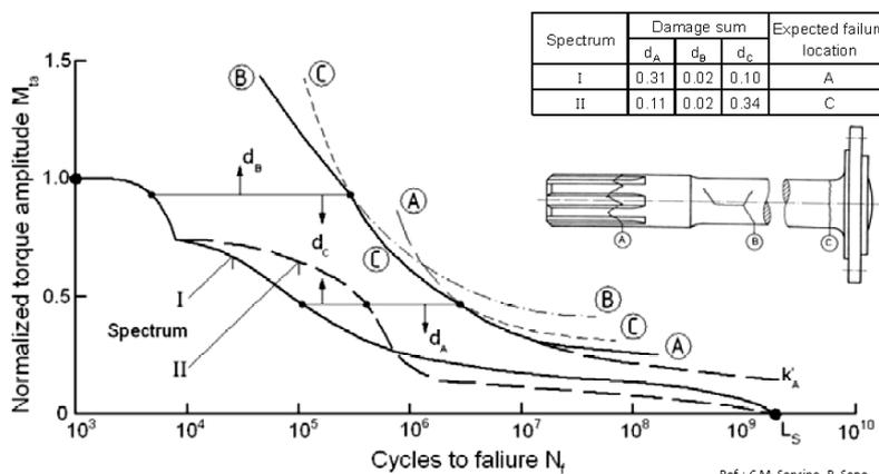
Figure 18. Failure sites of a driving shaft under constant and variable amplitude loading.
