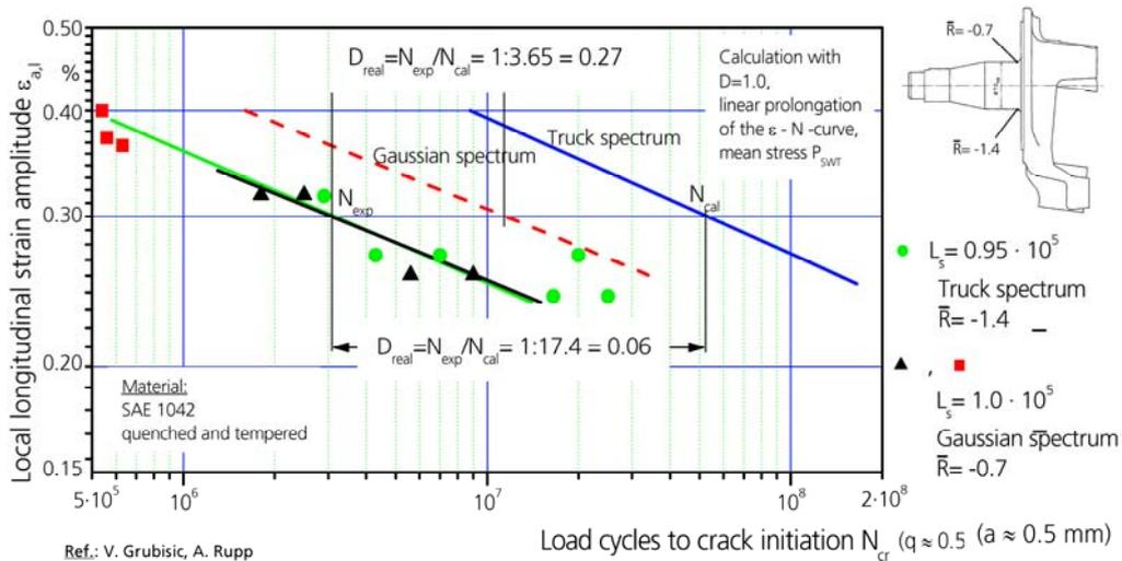
Figure 10. Experimental and calculated Gassner-lines, /10/.
