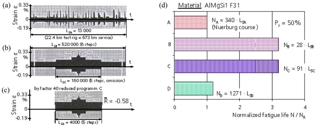
Figure 15. Influence of load mixing on variable amplitude fatigue life. (a) Original local strain-time history (A). (b) Blocked programs (B). (c) Sub-block programme (C). (d) Fatigue lives, /21/.
