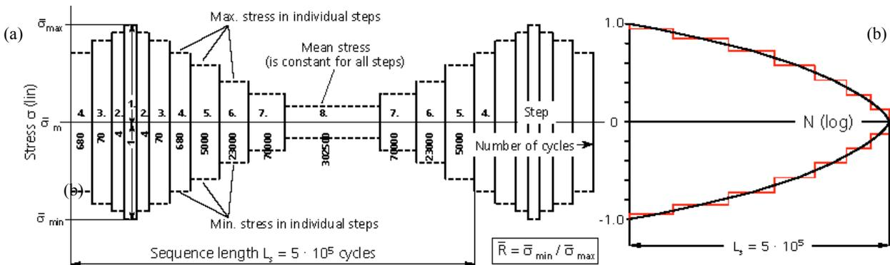
Figure 2. Ernst Gassner's historical 8 step-blocked-programme-sequence (1939). (a) Load sequence; (b) Cumulative frequency distribution.
