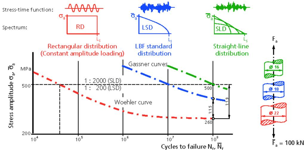
Figure 3. Influence of spectrum-shape on fatigue life and component dimensions.
