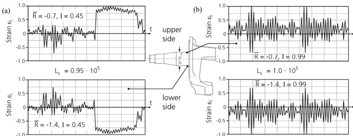
Figure 7. Applied local strain-time histories on a stub-axle and failure locations. (a) Truck strain-time history; (b) Gaussian strain-time history.
