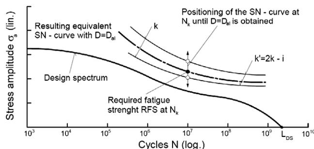
Figure 17. Determination of spectrum equivalent SN-curve for constant amplitude testing.
