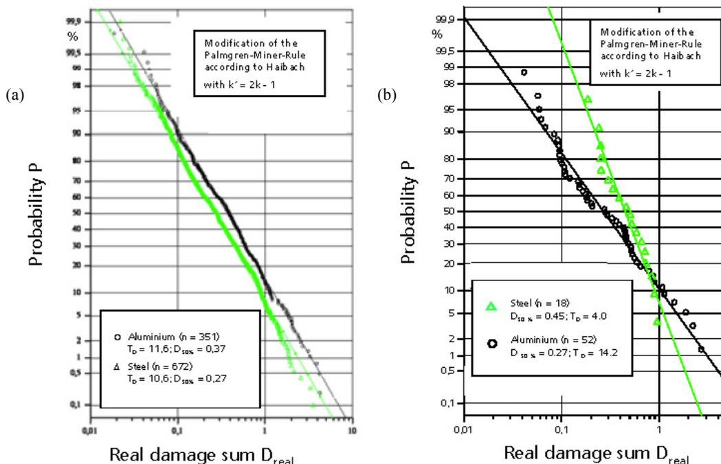
Figure 6. Real damage sum distribution for steels and aluminium alloys. (a) not welded; (b) welded joints, /9/.
