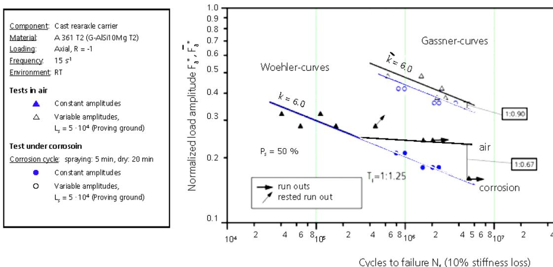
Figure 24. Fatigue strength of cast rear axle carriers in air and under corrosion.
