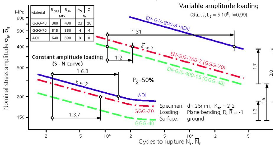
Figure 12. Fatigue behaviour of different cast iron materials under constant and variable amplitude loading.
