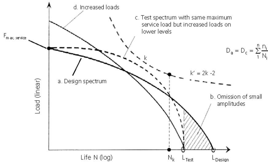
Figure 26. Possibilities for reduction of testing time, /31/.
