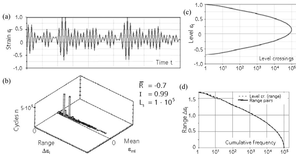
Figure 9. Gaussian load sequence. (a) strain–time history; (b) rainflow matrix; (c) level crossing counting; (d) level crossings and range pairs.
