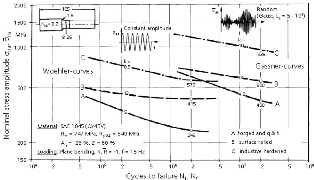
Figure 20. Influence of surface treatments on fatigue life of SAE 1045 axles under constant and variable amplitude fully reversed bending.
