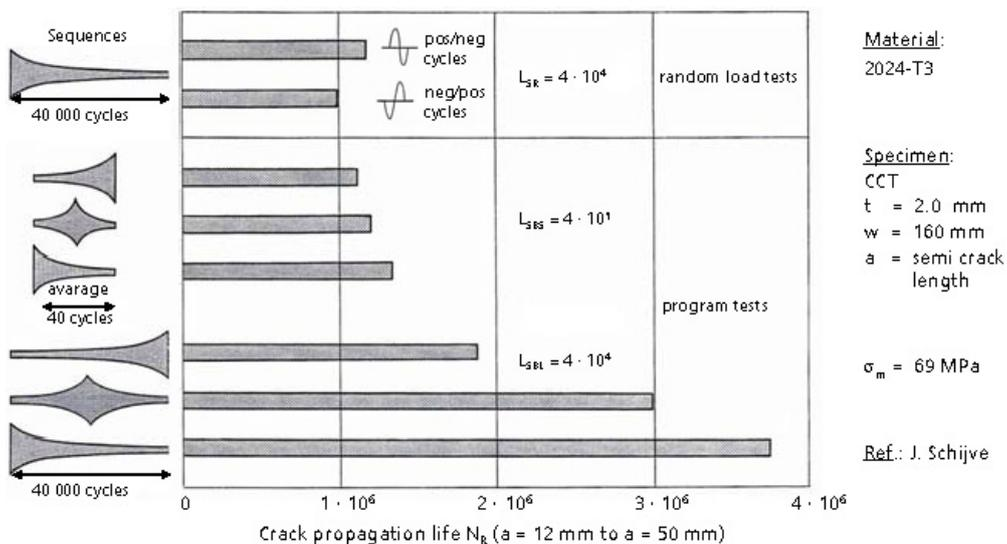
Figure 16. A comparison of fatigue crack growth lives under random loading and different types of programme loading by a gust load spectrum, /16/.
