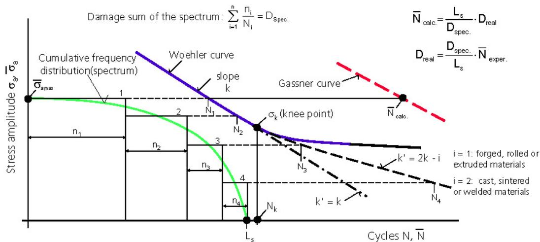
Figure 5. Most commonly used cumulative damage calculation methods.
