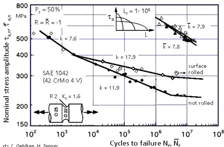
Figure 21. Influence of surface rolling on fatigue life of SAE 1042 axles under constant and variable amplitude fully reversed torque.
