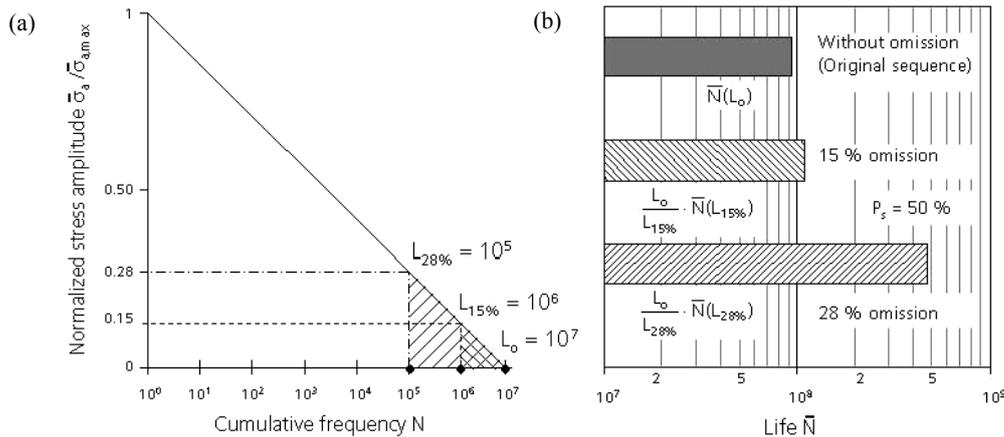
Figure 27. Influence of different omission levels on fatigue life. (a) Amplitude distribution, (b) Fatigue life.
