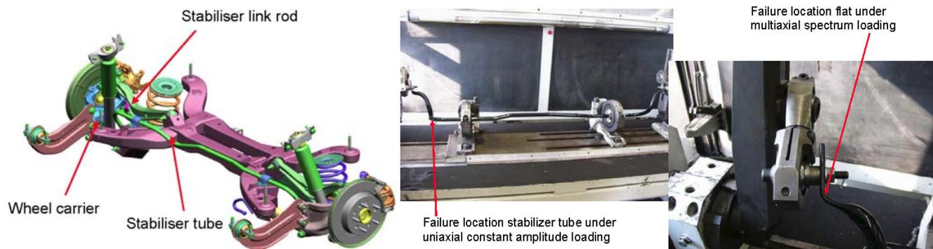
Figure 19. Rear axle stabilizer system with short link rods.
