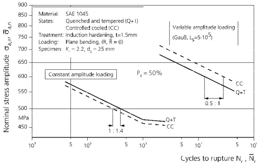
Figure 11. Woehler- and Gassner-lines of induction hardened steel variants.
