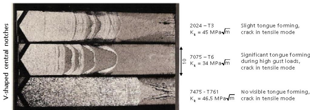
Figure 13. Material influence on crack front formation under variable amplitude loading, /15/.
