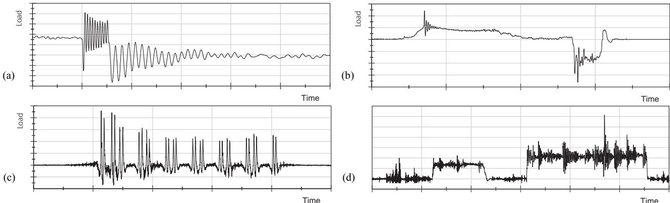
Figure 4. Examples of measured load-time histories: (a) wind energy plant, planet carrier, *special loading event*; (b) passenger car, trailer coupling loads (*acceleration, braking*); (c) rail loads during train crossing; (d) fork lift truck service loads.
