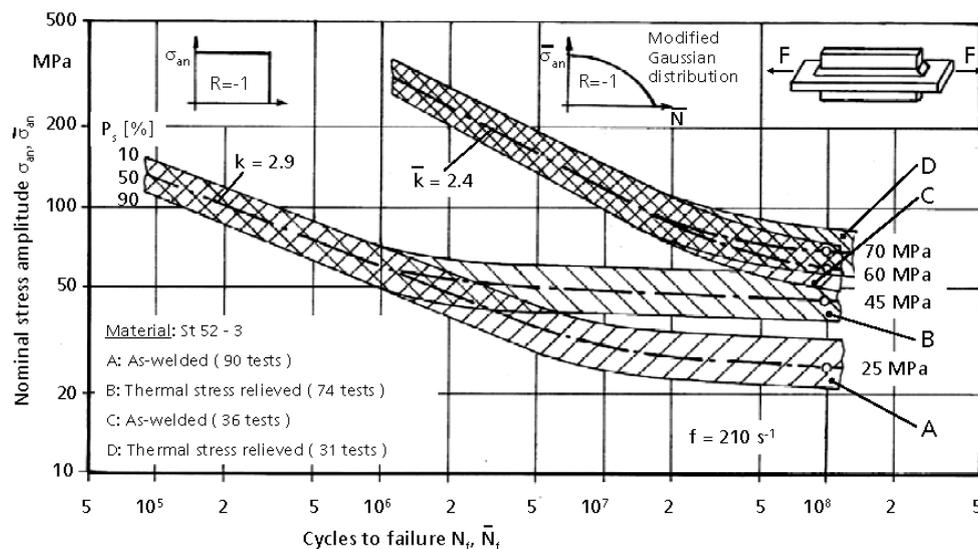
Figure 22. Fatigue life curves under constant and variable amplitude loading.
