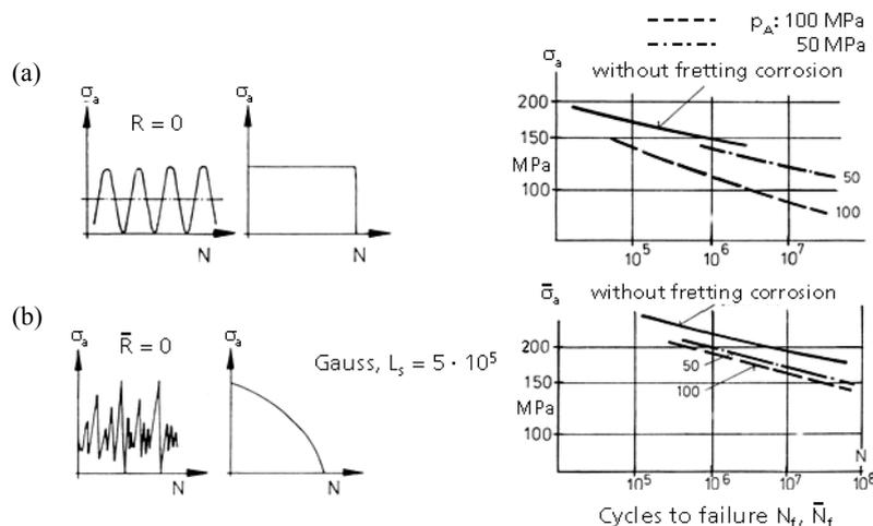
Figure 25. Influence of fretting corrosion and surface pressure on fatigue strength of a cast nodular iron. Material: EN-GJS-400-15
