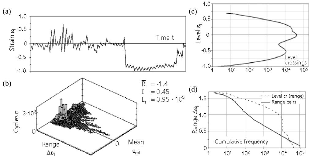
Figure 8. Truck load sequence. (a) strain–time history; (b) rainflow matrix; (c) level crossing counting; (d) level crossings and range pairs.
