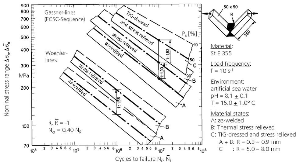
Figure 23. Fatigue behaviour of V-shaped specimens under constant and variable amplitude loading.
