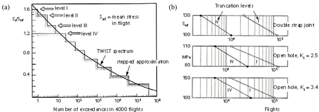
Figure 28. Effect of truncation of the TWIST load spectrum on fatigue life. (a) Stress amplitude distribution of the TWIST load spectrum, (b) Truncation levels and test results, /16/.
