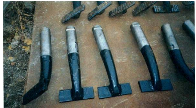
Figure 3. A lot with the old model of tamping tools type BNRI 85. Slika 3. Skup starih modela alata za nabijanje tipa BNRI 85
