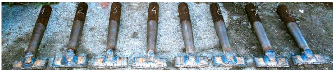
Figure 6. A lot with the old model of tamping tools type BNRI 85 Slika 6. Skup starijih modela alata za nabijanje tipa BNRI 85
