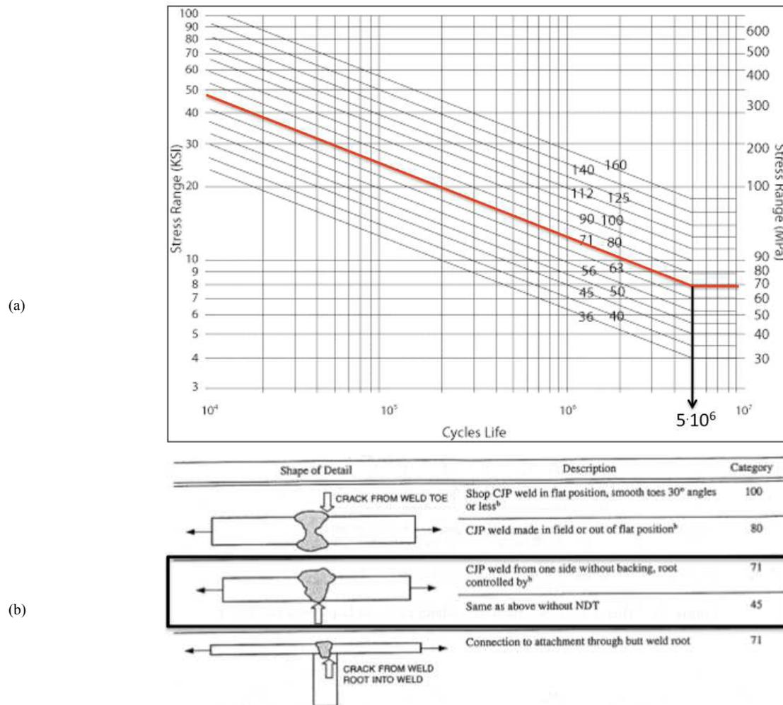
Figure 3. a) Fatigue strength curves for titanium welded joints from AWS D1.9 2007; b) detail categories for titanium alloys according to AWS D1.9 2007 (the detail of the present study is highlighted in the black frame).
