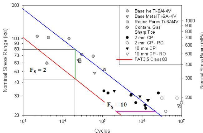
Figure 4. Derivation of fatigue design curves for welded titanium joints /6/.
