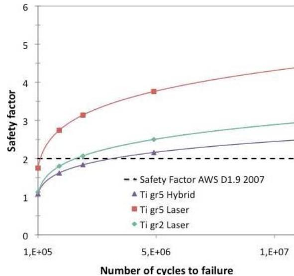
Figure 5. Safety factors for laser welded titanium grade 2 and 5 and for hybrid welded titanium grade 5 joints.
