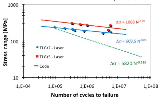
Figure 1. Fatigue resistance curves for laser welded grade 2 and grade 5 titanium alloys.
