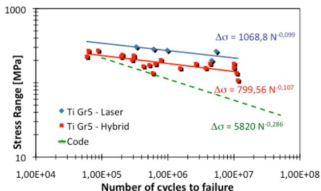
Figure 2. Fatigue resistance curves for laser and hybrid welded grade 5 titanium alloy.
