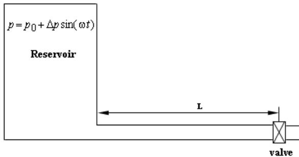
Figure 2. Installation of the resonant pipe.
