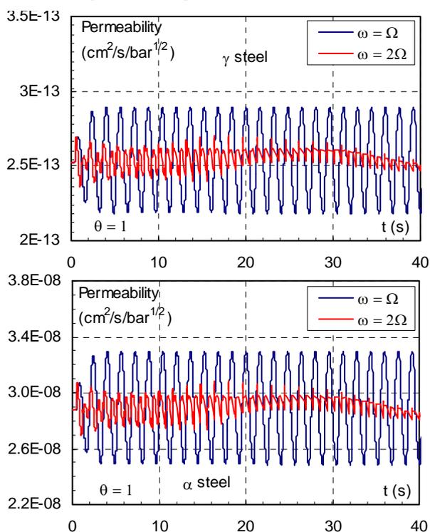
Figure 9. Permeability evolution in case of hydrogen ( $\theta = 1$ ), for frequencies  $\omega = \Omega$  and  $\omega = 2\Omega$ , for  $\alpha$  and  $\gamma$  steels.
