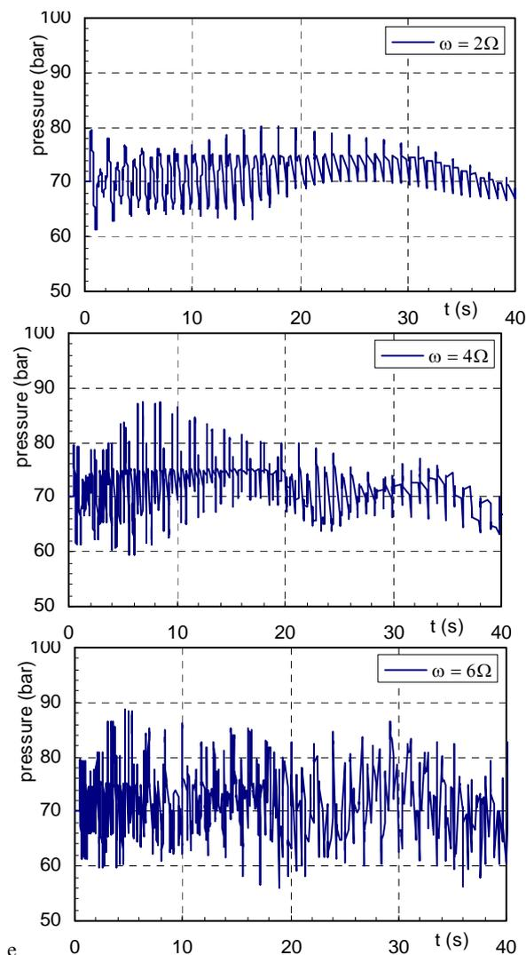
Figure 5. Pressure evolution for even frequencies at downstream end of pipe, for  $\theta = 1$ .
