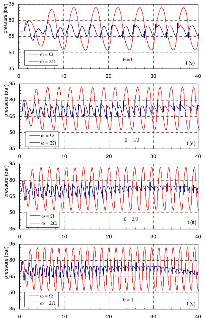
Figure 3. Pressure evolution for frequencies  $\omega = \Omega$  and  $\omega = 2\Omega$  at closed valve side, for different values of  $\theta$ .
