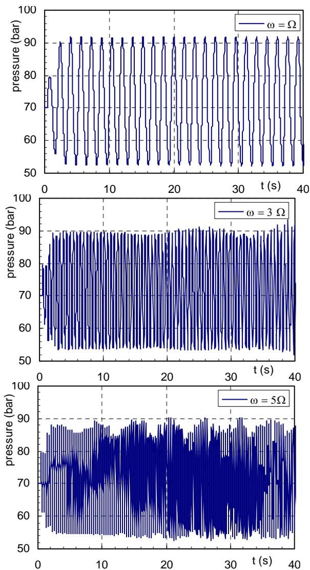
Figure 4. Pressure evolution for odd frequencies at downstream end of pipe, for  $\theta = 1$ .
