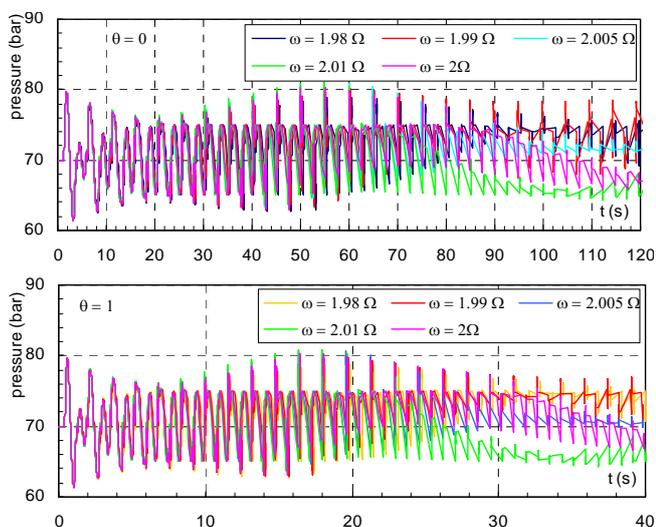
Figure 6. Pressure evolution in the neighbourhood of  $\omega = 2\Omega$  at the downstream end of pipe, for hydrogen mass fraction  $\theta = 0$  and  $\theta = 1$ . Slika 6. Razvoj pritiska u okolini  $\omega = 2\Omega$  na nizvodnoj strani cevi, za maseni udeo vodonika  $\theta = 0$  i  $\theta = 1$ .
