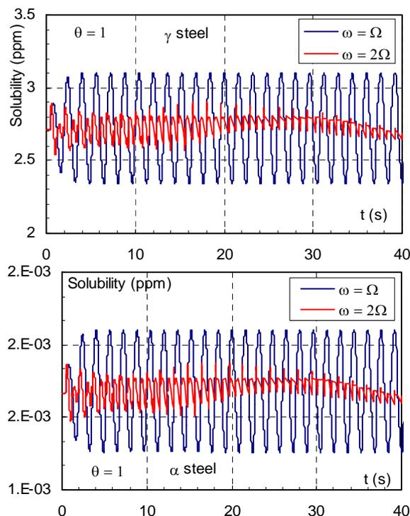
Figure 8. Solubility evolution in case of hydrogen ( $\theta = 1$ ), for frequencies  $\omega = \Omega$  and  $\omega = 2\Omega$ , for  $\alpha$  and  $\gamma$  steels. Slika 8. Razvoj rastvorljivosti za slučaj vodonika ( $\theta = 1$ ), za frekvencije  $\omega = \Omega$  i  $\omega = 2\Omega$ , za  $\alpha$  i  $\gamma$  čelike
