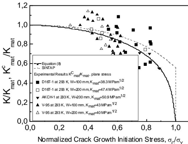
Figure 1. Comparison of predicted and experimental results of the failure assessment diagram at crack growth initiation for aluminium alloy centre-cracked tensile specimens at 293 K.
