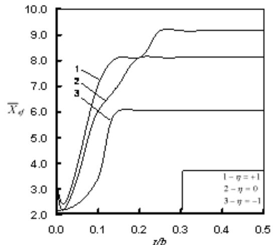
Figure 2. Distribution of the effective distance along the through-thickness crack front.
