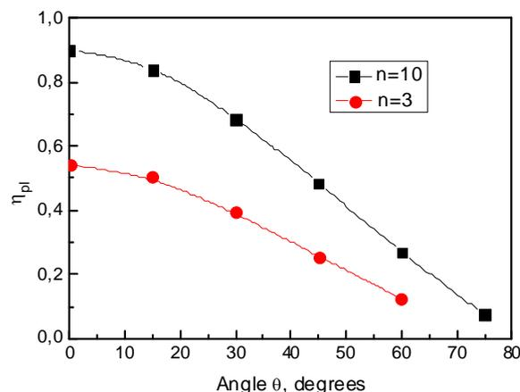
Figure 3. Mixed mode plastic factors for the tension plate with an inclined centre crack for power law hardening material.
