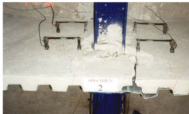
Figure 7. Specimen SP2, collapse of reinforced concrete. Slika 7. Uzorak SP2, kolaps armiranog betona
