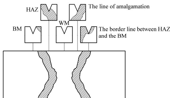
Figure 6. Notch position in relation to the welded joint.
