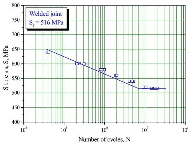
Figure 3. S-N diagramme for welded joint specimens.
