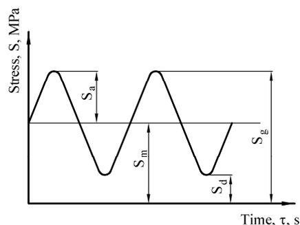
Figure 1. Alternating load scheme for stress ratio  $R = -1$ .
