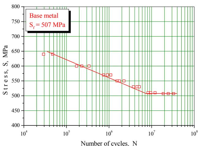
Figure 4. S-N diagramme for base metal specimens.
