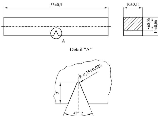
Figure 5. Specimen for impact energy determination.
