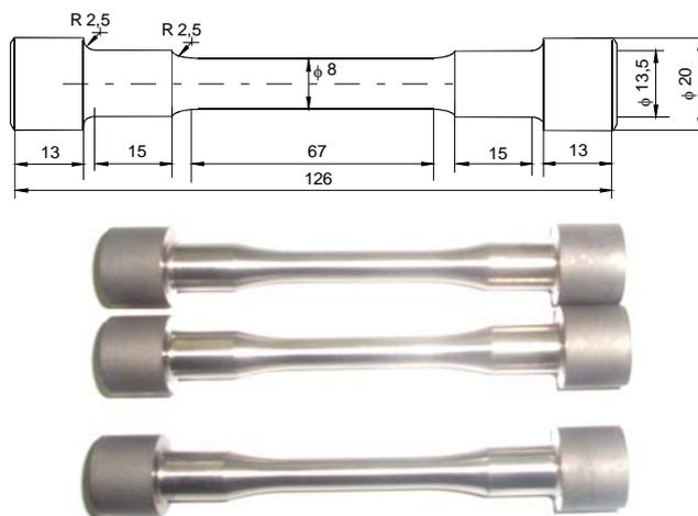
Figure 2. Fatigue test specimen design and view.
