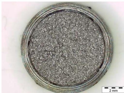
Figure 11. Fracture surface at  $-115^{\circ}\text{C}$  of notched tensile specimen quenched in water from  $1250^{\circ}\text{C}$ .
