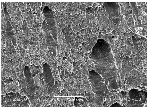
Figure 8. Shearing ductile decohesion at 22°C.
