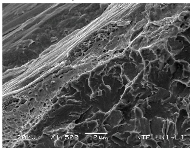
Figure 12. Details of the shearing ring at notch tip of notched tensile specimens fractured at  $-115^{\circ}\text{C}$ .
