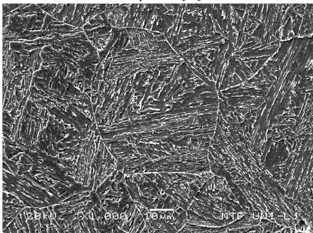
Figure 3. Microstructure after lead bath cooling from 1250°C.
