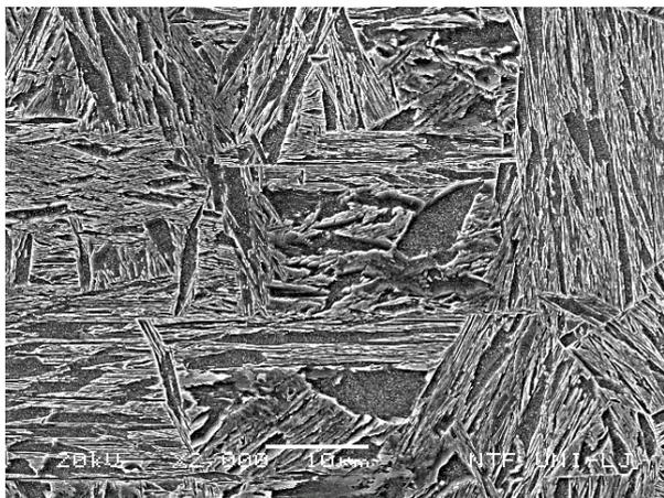
Figure 1. Microstructure after water quenching from 1250°C.
