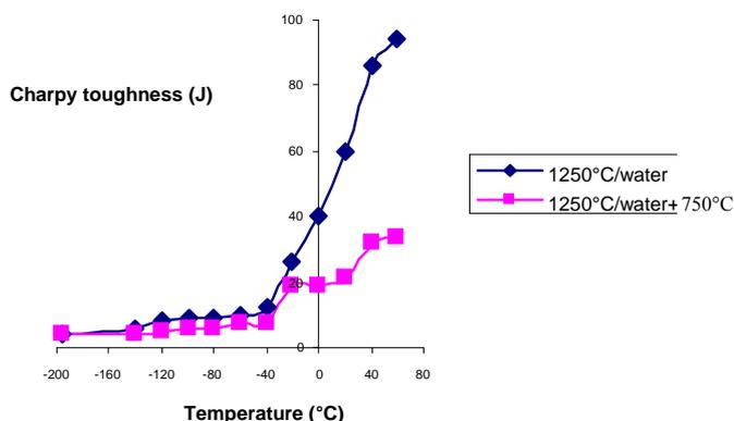
Figure 5. Charpy toughness versus testing temperature for the steel quenched in water from 1250°C and reheated.
