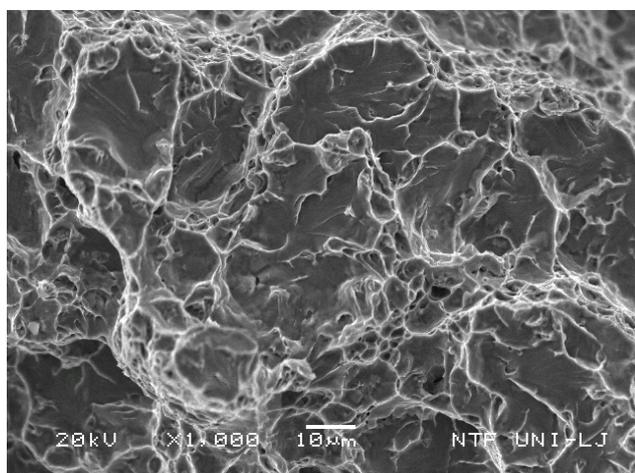
Figure 9. Fracture at 0°C of steel quenched in water from 920°C.
