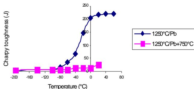
Figure 6. Charpy toughness versus testing temperature for the steel cooled from 1250°C in lead bath and reheated.
