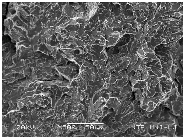
Figure 10. Fracture at -60°C of steel quenched in water from 920°C.
