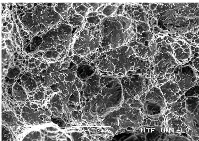
Figure 7. Normal ductile decohesion at 22°C.
