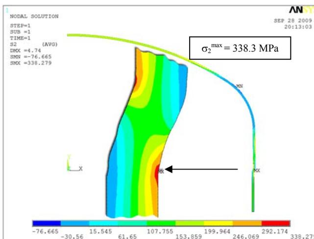
Figure 11. Principal stress  $\sigma_2$  distribution ( $e = 8$  mm).
