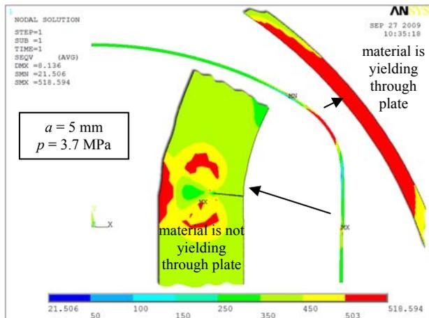
Figure 15. Material yielding in pressure vessel head, but not in the area around the crack.
