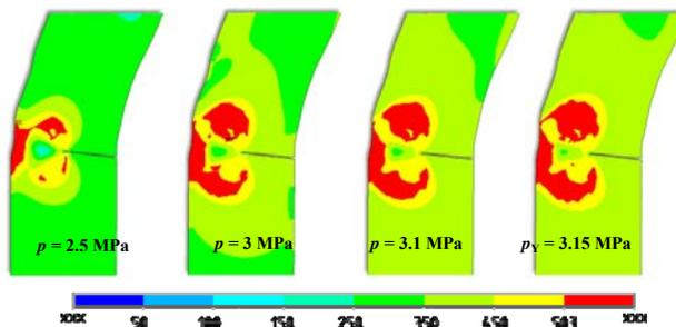
Figure 18. Material yield spread,  $a = 7$  mm.
