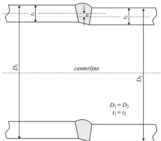
Figure 1. Centreline offset weld misalignment.
