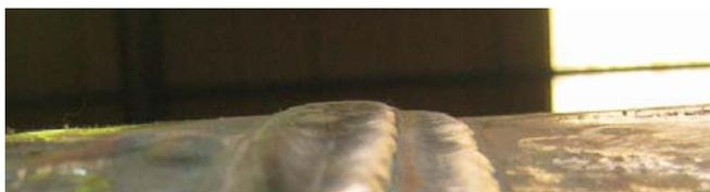
Figure 2. Weld misalignment in the vessel body.
