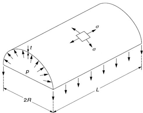
Figure 12. Stress directions in an cylindrical pressure vessel.
