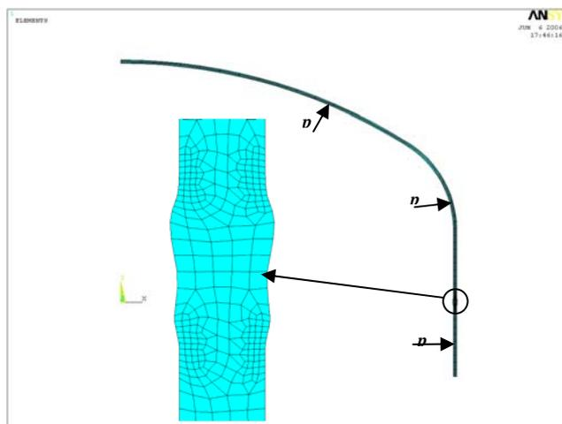
Figure 5. Finite element model of the vessel.
