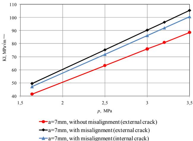
Figure 19. Stress intensity factor variation due to different pressure values ( $a/t = 0.5$ ).
