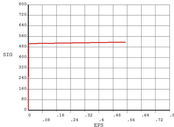
Figure 9. Linear elastic-ideal plastic material.
