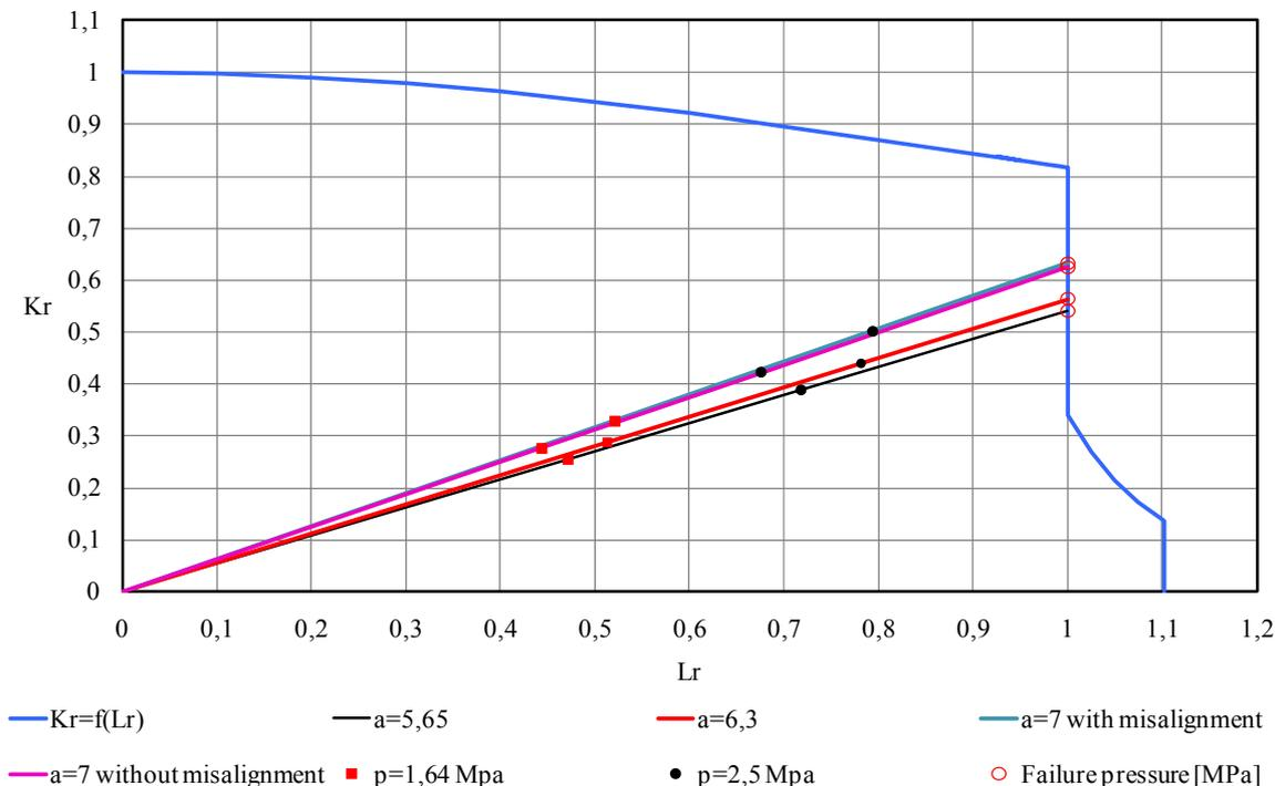
Figure 20. Failure assessment diagram (FAD diagram).
