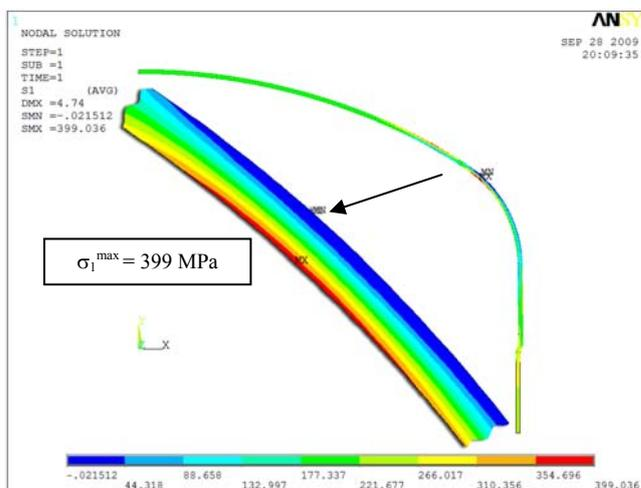
Figure 10. Principal stress  $\sigma_1$  distribution ( $e = 8$  mm).
