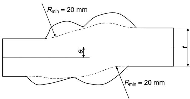
Figure 8. Roundness of the welded joint.
