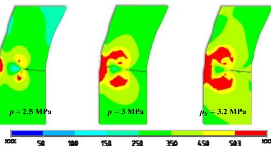
Figure 17. Material yield spread,  $a = 6.3$  mm.
