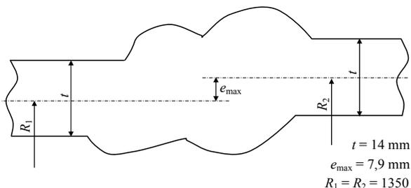
Figure 4. Geometry of weld misalignment.
