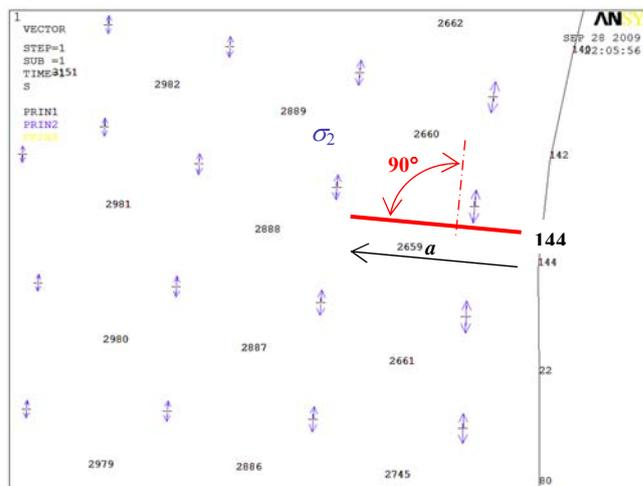
Figure 14. Crack will appear perpendicular to the vector of maximal principal stress  $\sigma_2$ .
