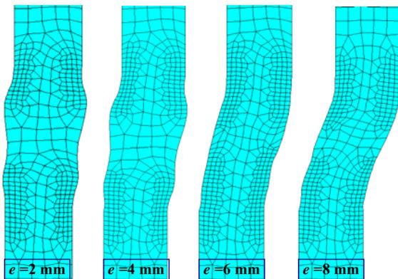
Figure 7. Finite element models for weldments of various misalignments.
