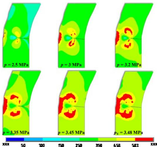
Figure 16. Material yield spread,  $a_{min} = 5.65$  mm.
