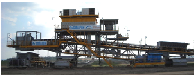
Slika 6. Izgled jednog realizovanog tračnog transportera sa regulisanim pogonom 4 \times 1,2 MW u sklopu V BTO sistema Figure 6. The exterior of one realized belt conveyor with controlled 4 \times 1.2 MW as a part of the 5th BSC system.
