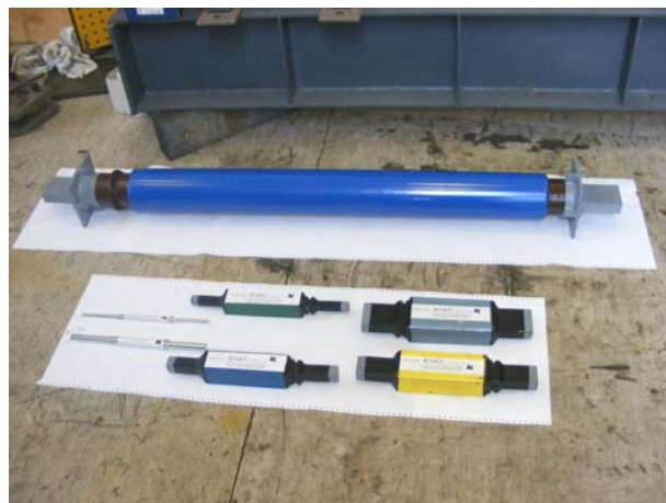
Figure 16. Typical damper for bridge application, tested at VTI. Slika 16. Tip dampera za primenu na mostu, ispitan u VTI
