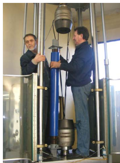
Figure 17. Testing of one sample of damper "Bridge", nominal length l = 1000 mm, at Military Technical Institute (VTI). Slika 17. Ispitivanje uzorka dampera „Most“ nazivne dužine l = 1000 mm u Vojnotehničkom institutu (VTI)
