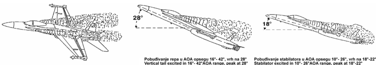
Slika 7. Bafting repa pri visokim AOA Figure 7. Empennage buffet at high AOA.
