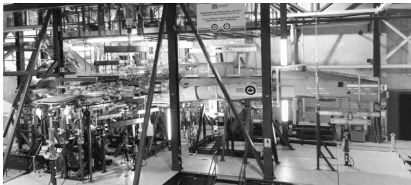
Slika 3. CF-18 IFOSTP ispitivanje na zamor centralnog dela trupa (FT55) u prirodnoj veličini u laboratoriji Bombardir (sada L3) Figure 3. CF-18 IFOSTP Centre Fuselage Full Scale Fatigue Test (FT55) at Bombardier Aerospace Defence Services (now L3).
