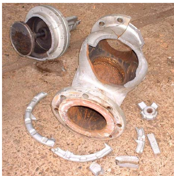
Figure 10. Isolation valve ruptured by the condensate slug impact. Slika 10. Pregradni ventil slomljen zbog udara čepa kondenzata
