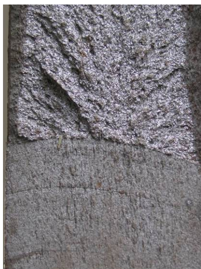
a) Transition from fatigue to stable crack growth, shear lips visible (IP) b) Extend of crack till formation of first final stretch zone (CA) c) Second final stretch zone (ZP) before final brute fracture
