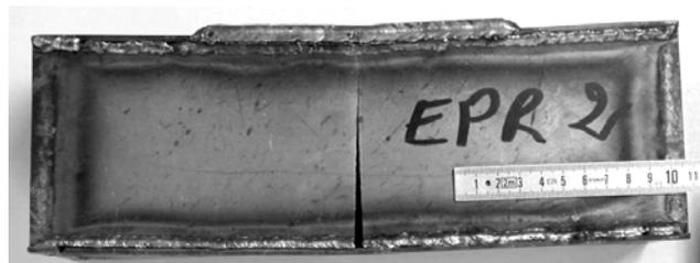
Figure 8. Fracture of box specimen in fatigue bending test.
