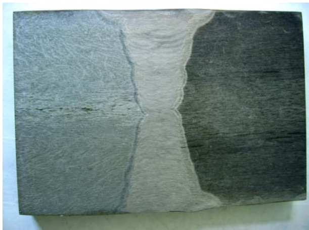
Slika 5. Makrosnimak zavarenog spoja Figure 5. Macrograph of welded joint.
